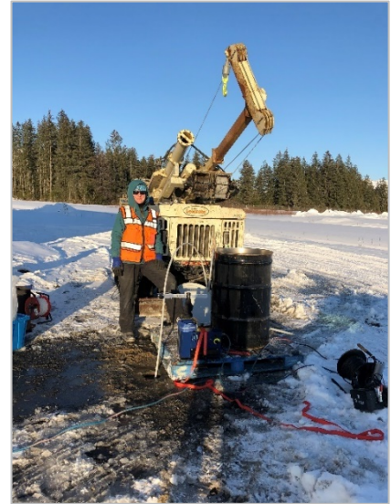
Exhibit 3-3: Well development at MW-3 using a Waterra inertial pump.
