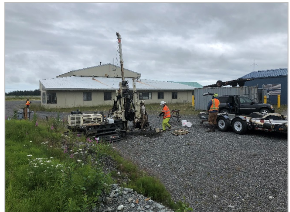
Exhibit 2-1: Advancing a geotechnical soil boring in July 2020. Photo taken facing south.
