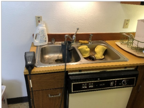
Exhibit 3-6: Monitoring water quality parameters using a YSI while purging the ARFF existing water supply well.
