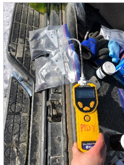
Exhibit 3-1: Field staff conduct headspace field screening of soil using a PID.
