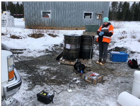
Exhibit 3-4: Field staff fill drums with purge water from MW-4. Photo taken facing north (left). Monitoring water quality parameters using a YSI while purging TWP-6 (right).
