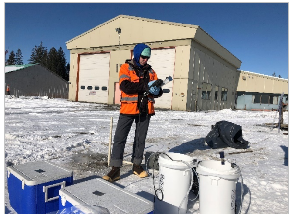
Exhibit 3-4: Field staff fill drums with purge water from MW-4. Photo taken facing north (left). Monitoring water quality parameters using a YSI while purging TWP-6 (right).
